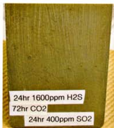
Gaseous environment test panel. Low-VOC rust-converting water-based primer and high-solids moisture-cure urethane coating, 4.2 to 4.5 mils DFT.
